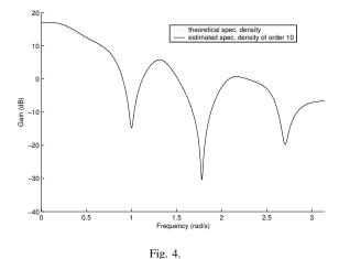
n = 10 estimate of spectral density together with the true spectral density.
