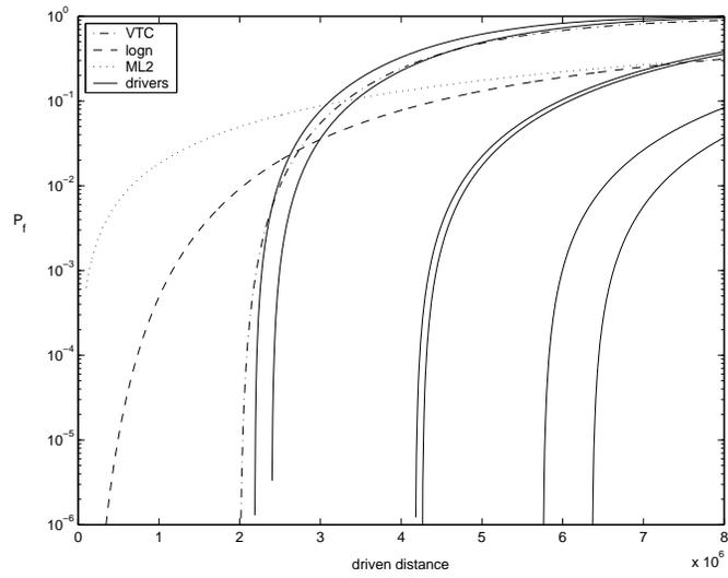
Figure 4.8: Failure probability  $P_f$  for different  $s$ , Highway.
