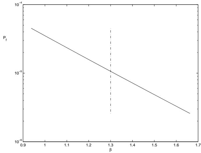
Figure D.2: Failure probability  $P_f$  for different  $\beta$ , varying around  $\beta = 1.30$
