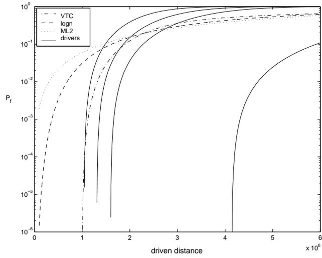
Figure 4.7: Failure probability  $P_f$  for different  $s$ , City.
