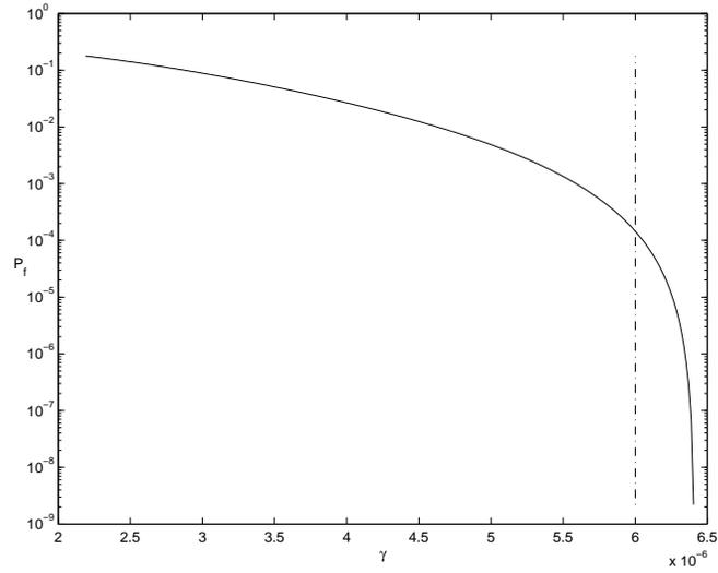
Figure D.5: Failure probability  $P_f$  for different  $\gamma$  when  $\beta = 0.65$
