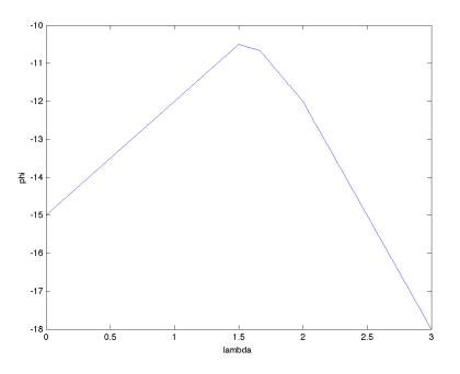
The figure gives  $\lambda^* = 1.5$  with  $\varphi(\lambda^*) = -10.5$ . By inspection one can see that the optimal solution to (KP) is given by  $x^* = (1 \ 0 \ 1)^T$  with  $c^T x^* = -9$ . The duality gap is therefore 1.5.
