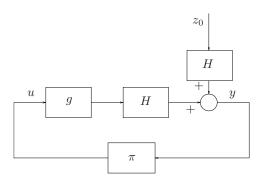
Fig. 3. An equivalent feedback configuration.
