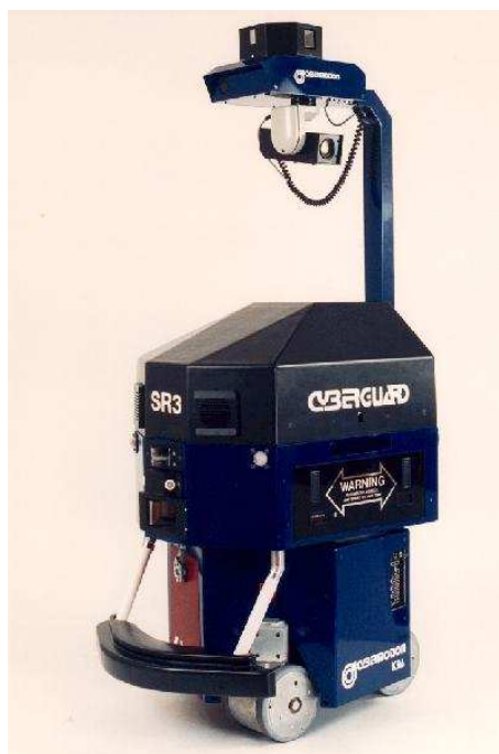
Figure 3.2: The CyberGuard SR3 based on the K3A platform. Image courtesy of Cybermotion Inc.
