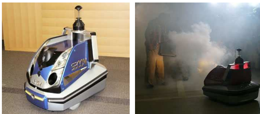
(a) Since 2005, Secom's six-wheeled sentry vehicle, Robot X, can be rented for a price of 2600$ per month. (b) The smokescreen of Robot X is meant to frighten off, or at least confuse, the intruder.
