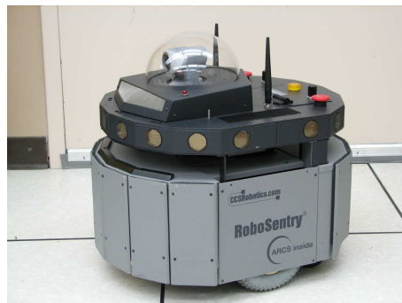
Figure 3.6: RoboSentry Defender is a derivative product built upon the PatrolBot platform, Image courtesy of CCS Robotics.
