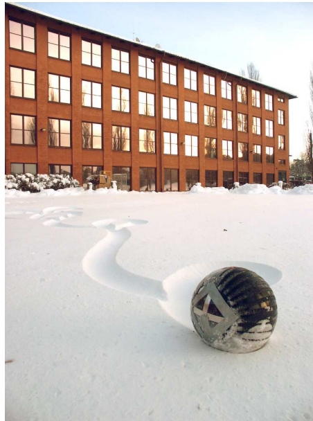
Figure 3.3: Rotundus' spherical robot handles rough outdoor environments elegantly. Image courtesy of Rotundus AB.
