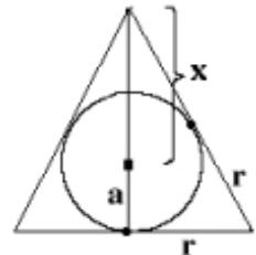
$$\text{Cone volume } V = \frac{\pi r^2 h}{3} = \frac{\pi}{3} a^2 \frac{x + a}{x - a} (x + a) = \frac{\pi a^2}{3} \cdot \frac{(x + a)^2}{x - a}.$$
