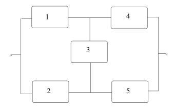
In the system above the life lengths of the components are associated and hence their state variables are associated at each time. All components have the failure rate  $\lambda$ .
