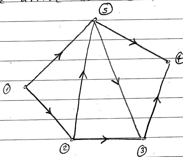
Also from b, we see that nodes ①, ② are source nodes with supplies 5, 5, respectively, while nodes ③, ④, ⑤ are sink nodes with flows 4, 3, 3, respectively going out of the network. So we have:
