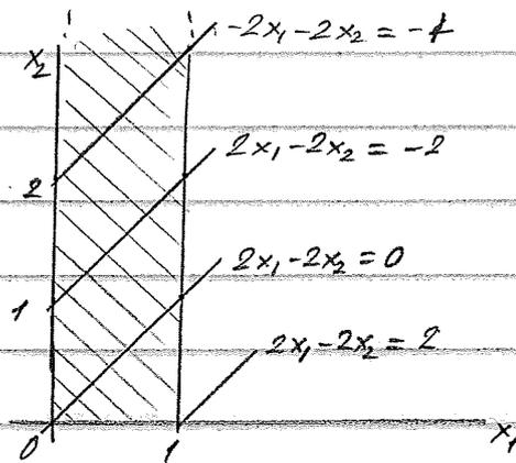
There is no optimal solution, and the optimal value of (P) is  $-\infty$ . (For example,  $x_n = \begin{bmatrix} 0 \\ n \end{bmatrix}$ ,  $n \in \mathbb{N}$ , are all feasible, and  $c^T x_n = 2 \cdot 0 - 2 \cdot n = -2n \rightarrow -\infty$  as  $n \rightarrow +\infty$ .)
