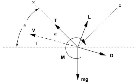
FIGURE 1. Variables for the aircraft model.
